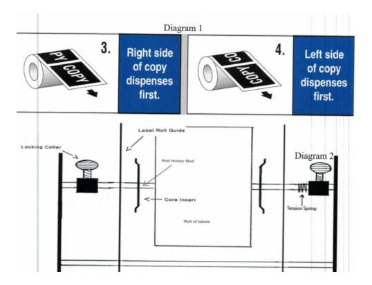
There are two 1 " long, 1/16" aluminum roll guides and a tension spring included with the machine. These guides should be placed on either side of the roll of labels between the metal core inserts and the locking collar. The notches on the end of the guide slide onto the chrome rod at the bottom of the machine. Tension spring goes between the right roll guide and the locking collar on the right side of the roll of labels as shown in diagram 2.
