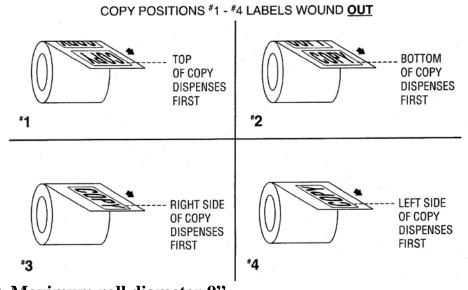
4.) Maximum roll diameter 9" \*Upgrade to 15" diameter for \$35
