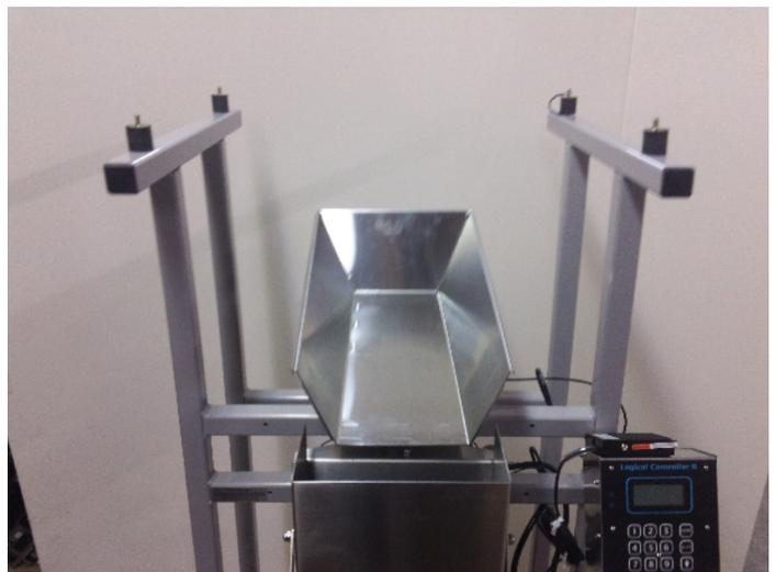
Fig. 2: Feed Pan exposed after removing Supply Hopper
