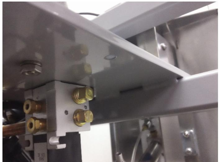
Fig. 7: Solenoid and chassis without air hoses attached
