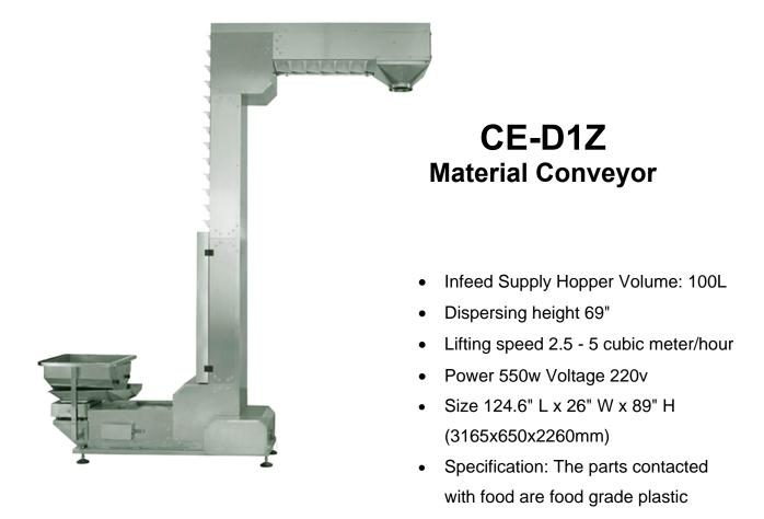
The CE-D1Z conveyer is appropriate for vertical lifting of granule material, for example, corn, grain, plastic and granule applications, and so forth. The container is moved by the conveyor chains. Utilized for vertical dispensing of granules or small piece material. the CE-D1Z can handle large amounts lifting to 69" max. All parts contacted with food are food grade plastic.
