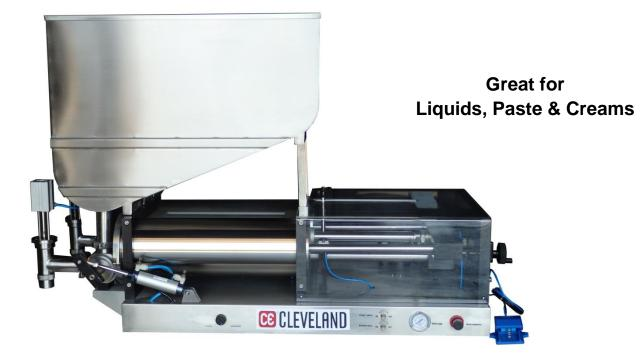
The Cleveland Equipment SGP-D series piston filler is a dual head bench-top piston filler that offers additional production output. This non-electric piston filler is operated with a foot pedal that triggers the fill cycle, making it great for use in wet or damp environments or anywhere that isn't wired for electricity. All touch materials of this machine adopt 316 stainless steel,
