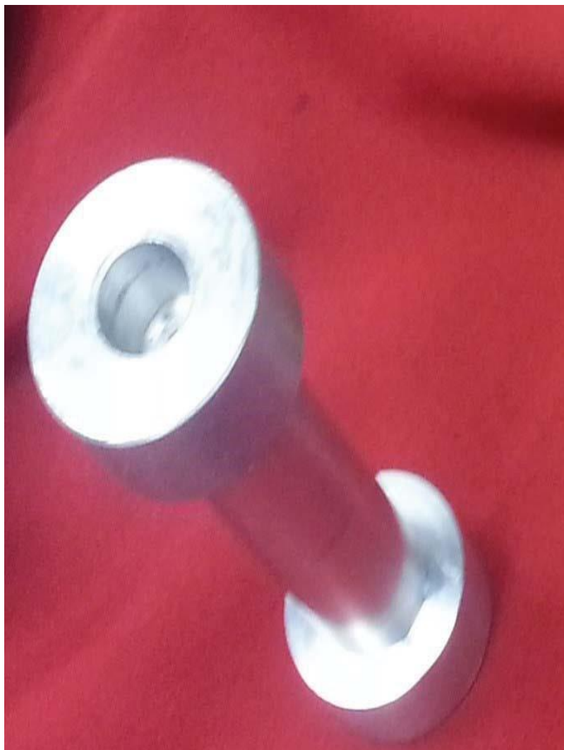
The bearing shaft driver DO NOT hit directly on the shaft us this tool
