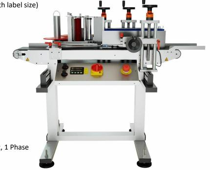
The Inline Automatic Wrap-around Labeler is perfect for adhering a label around your cylindrical bottle. Simple to use with Quick and simple product changeover. Motorized conveyor and wrap belt with speed control. Integrated control panel for easy adjustment. Accurate Optical fiber sensor and precise label dispensing.
