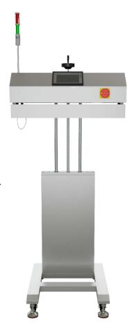
The Continuous Duty Air-Cooled Induction Sealing Machine is a contact-less cap sealing system to hermetically seal the top of plastic and glass containers with foil seals providing secure tamper evidence, preserve freshness, and prevent leakage. This sealing process takes place after the container has been filled and capped. The sealing head is adjustable and can be skewed to reduce exposure time, if necessary.
