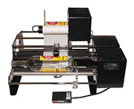
For labeling cylindrical containers, front and back, from .5" to 6" Diameter.
