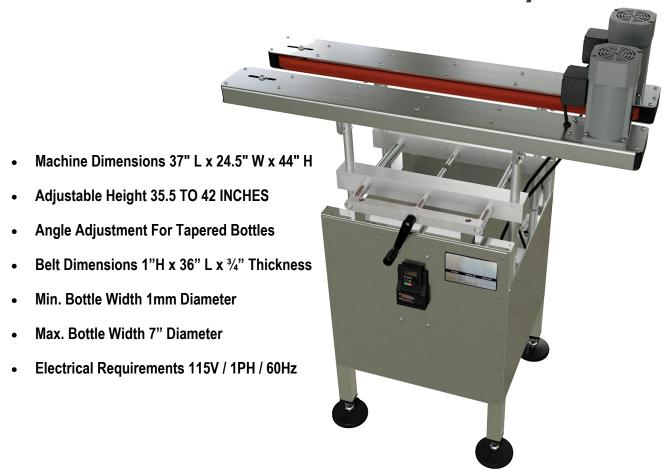
The CE-TRA-37B Bottomless Conveyor has variable speeds and is used in moving containers a short distance from one working/transportation conveyor to another. Designed to access the bottom side of the container for coding expiration dates, lot numbers, etc. The Gripper Belts are independently adjustable and can accommodate containers from 1 mm to 7" in diameter.
