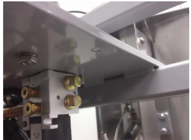
Fig. 7: Solenoid and chassis without air hoses attached
