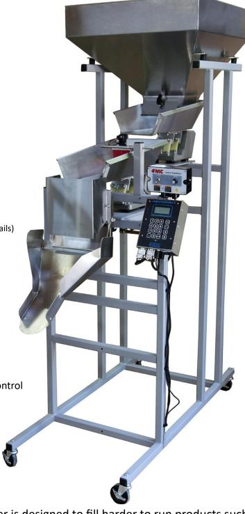
The CE-S6 Cascading Vibratory Linear Weigh Filler is designed to fill harder to run products such as crackers, chips and other non-free-flowing or irregularly shaped products. A very accurate and easy to use control system monitors the product depth in the lower pan allowing for consistent filling. The CE-S6 utilizes many of the same systems found on our CE-S4, including the Logical Controller II, for reliable, hassle free operation.
