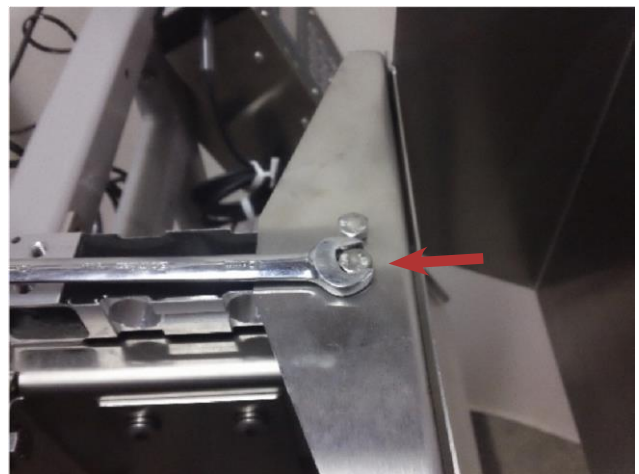
Fig. 8: Removing the two 10mm bolts holding the Weigh Hopper
