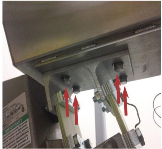
Fig. 3: (4) 5/16-18 bolts hold the Feed Pan to the Vibrator.
