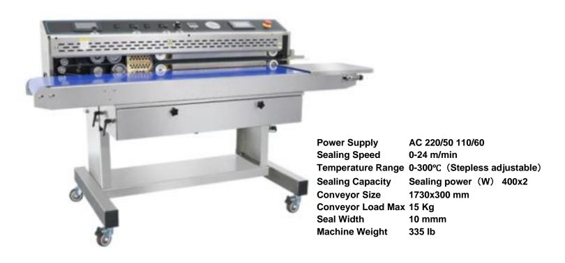
The CE-6800 Horizontal Sealer is suitable for sealing medium and large bags that require vacuum or flushing. It integrates vacuum, flushing, sealing and ink-jet coding. It adopts touch screen for the simple operation, multiple functions, and perfect sealing effect.
