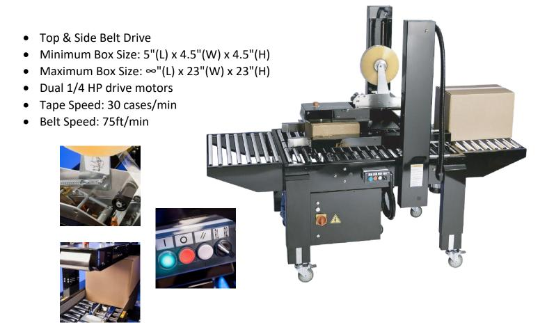
The SB-EX Random allows users to run a variety of case sizes without having to manually adjust for each box. The system's unique and simple design has proven to be one of the most reliable case tapers on the market today, keeping production and maintenance efforts to a minimum and providing fast and efficient alternatives to hand taping.
