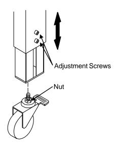
CAUTION! The case taper must be lifted off the floor to install the casters.
