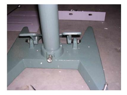
**Identify the base**. It will have four rubber pads for feet on the bottom of it. In one corner it will have an adjustable screw to allow for variations in floor level.
