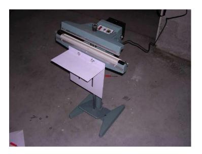
The final step is to install the work plates on the front of the unit. This can be done a couple of different ways. The way I recommend is to take the slotted faceplate and mount it to the front of the sealer using to the short hex bolts, lock washers and nuts. Then mount the 90-degree plate to the adjustable slots of the slotted plate using two of the short hex bolts, flat washers and nuts. The idea here is to allow you an adjustable platform to rest the product on while sealing.
