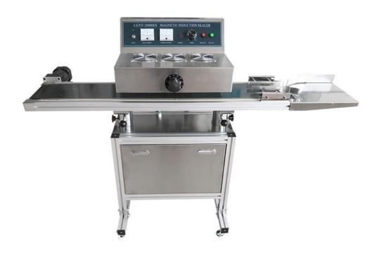
The CE-975 continuous induction sealer utilizes electro magnetic induction producing an instant high heat to melt aluminum foil that then adheres to the bottle opening. The CE-975 provides a wet-proof, leakage-proof, mildew-proof seal that also extends preservation time. Widely used as sealing package machine in industries such as pharmaceuticals, pesticides, pesticides, lubricant and cosmetics etc.
