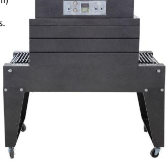
With durable Construction with easy operation and maintenance, the CE-215 heat shrink tunnel provides even heat distribution using Infrared Quartz Heating Tubes to surround your product. A Variable Conveyor with speeds 0-30ft/min, Teflon Curtains to keep the heat in, Circulation fan for even heat distribution. Distance between the rollers is 0.75 in.
