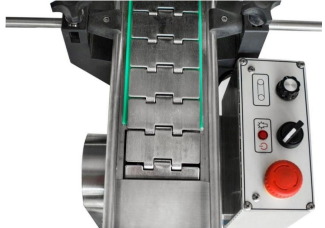
Stainless steel conveyor adjustable conveyor speed
