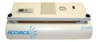
MAX Vacuum: 27 in HG. Air Consumption: 5 CFM @ 90 PSI Voltage: 120 VOLTS AC 7 amps.
